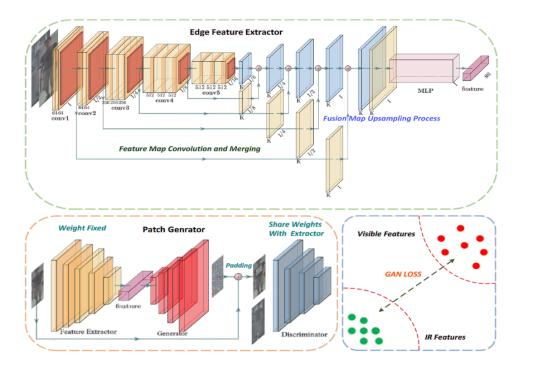
Thus, I developed a GANbased generative model for self-supervised, in-sample adversarial example generation. By using the semantic feature distance between adversarial and original samples as the evaluation metric, we completely bypassed model training. This approach achieved significant attack success on unseen pedestrian matching models.
