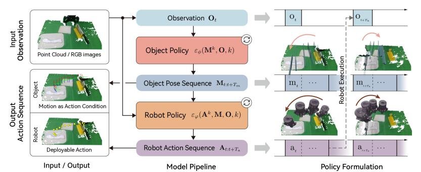
MBA is a cascaded diffusion framework. It predicts future object motion from observations, then uses this prediction to condition robot action generation. Leveraging pose consistency, MBA **avoids staged training unlike flow-based methods**. We jointly supervise object and robot poses, enabling end-to-end inference. Experiments also show MBA surpasses Flow-based methods in action generation, likely because it **avoids the 'vision-motion' gap** by directly modeling motion.
